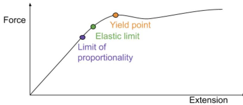
**Elastic deformation** is where a material **returns to its original shape** once the force applied is removed. This is because **all** the work done is stored as **elastic strain energy**.
