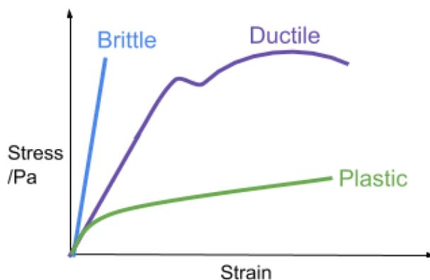
The **breaking stress** of a material is the value of stress at which the material will break apart, this value will depend on the conditions of the material e.g its temperature.
